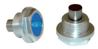
Consisting of a milled hexagonal head and crown in light aluminium alloy, the metal plug with magnet (which can also be used as a normal tank drain plug) can catch the metal particles present in the oil.
