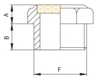
The silencer cap with sintered pad condenses the vapours present, making them fall back inside the tank.
