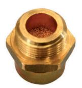
This range of oil breather caps has the same constructional characteristics as the TCSL, with the addition of a sintered bronze washer in the bottom part of the vent chamber, making it suitable for a "heavier duty" and therefore suitable for: reduction units, overdrives, building machinery, road machinery, etc.
